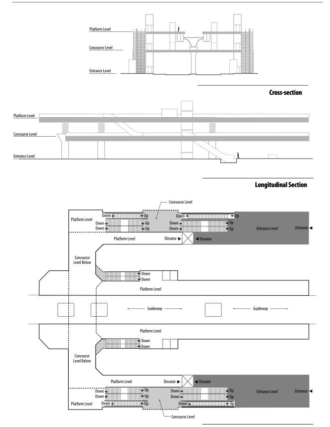
**Figure 2-14** Typical Side-platform Station Configuration with a Concourse
