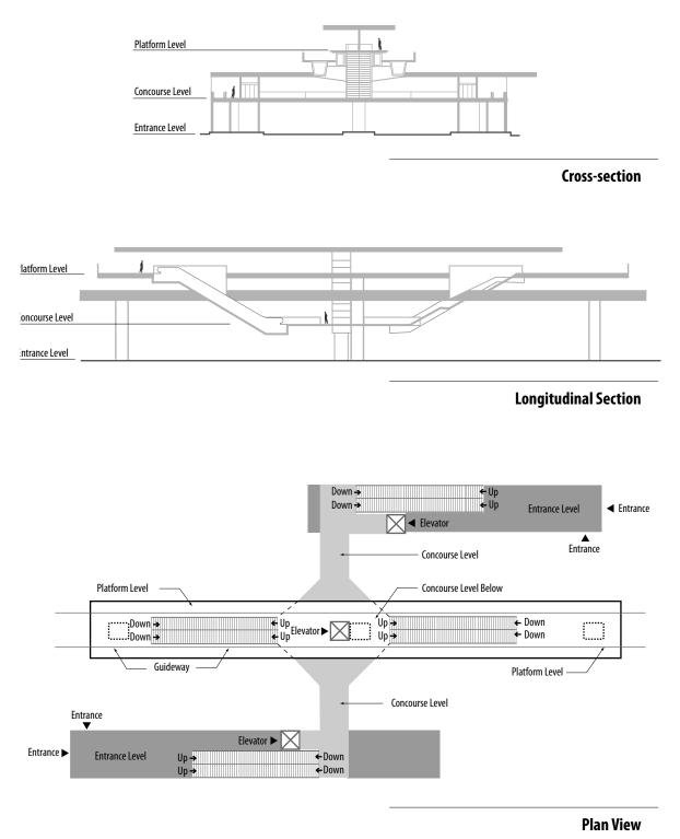
Figure 2-15 Typical Center-platform Station Configuration with a Concourse
