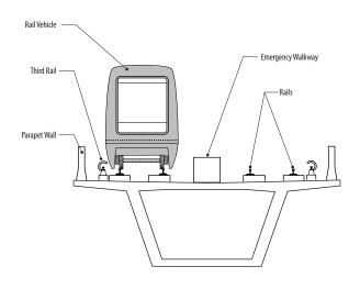
Figure 2-12 Example Vehicle on Elevated Guideway (Cross-section)
